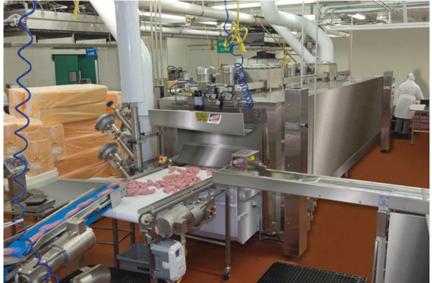
When the market for its al fresco brand chicken links took off faster than expected, Kayem Foods upgraded to a patented impingement freezer from Linde.
