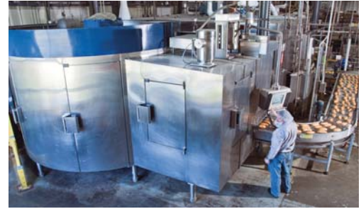
The Cryoline® XF spiral freezer features proprietary cross-flow technology for high-efficiency heat transfer.
